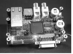
Fig. 2 FPGA board.
